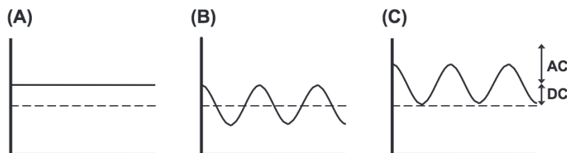
FIGURE 5.3 Different types of voltage variation. Dotted line = 0 V, solid line = signal. (A) DC offset, in which the signal has a steady deviation (in this case positive) from zero. (B) AC (alternating current) signal, which oscillates above and below zero. (C) AC signal, which oscillates above and below a constant DC offset.
