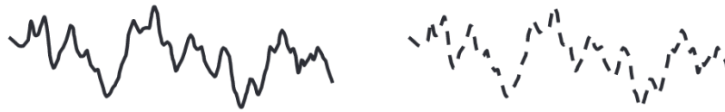
FIGURE 5.5 Neural signals are produced continuously (left) but must be sampled at intervals and converted to a sequence of numbers (right) by an A–D converter.
